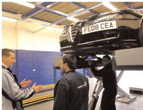
was key in reducing that 'Alfa wander' and livening up the initial turn in. Final settings from front and rear, gave a perfect zero on thrust angle and steer ahead, so the car would truly track straight, with the camber, caster and toe now working in harmony.
