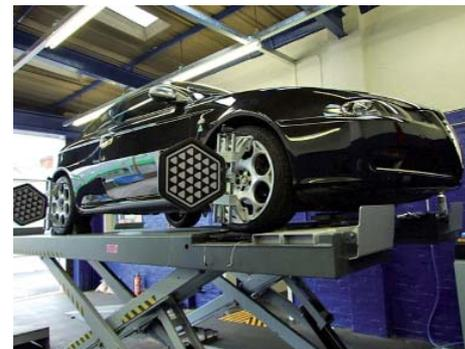
on steering feel. (Have I lost you? Me too nearly!). 'Toe' is the angle a wheel has in relation to its forward movement. The latter is what people often believe to be solely responsible for excessive tyre wear – excessive 'toe out' (commonly set at the factory on Alfas) wearing the inside edge, 'toe in' wearing the outside edge. Now, Peter is at pains to explain, it's not just toe that has effect on wear and steering response, it's the combination of all three factors.
