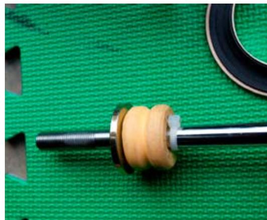
spring (gaining spring rate as it's compressed). "The more a MPU bumpstop is compressed, the progressively stiffer it gets. So if you compressed it half an inch, it may take 100 lbs of force. To compress it another half an inch may take 500 lbs of force. One would think that a bumpstop could just be made out of a simple block of this material and work well, and this is usually the case with a short one, say 2 inches or less. But longer ones tend to distort as
